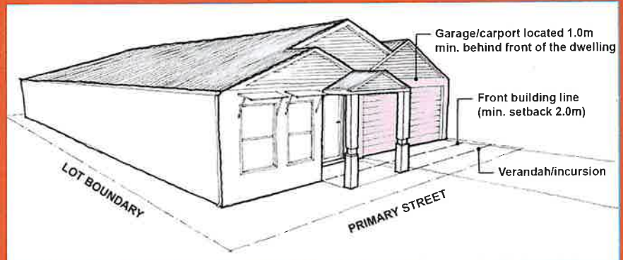
Fig. 11: R60 garages should be located behind the front building line of the home.
