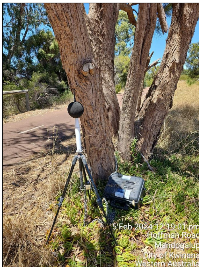
FIGURE 4.3 - NOISE MONITOR IN SITU
