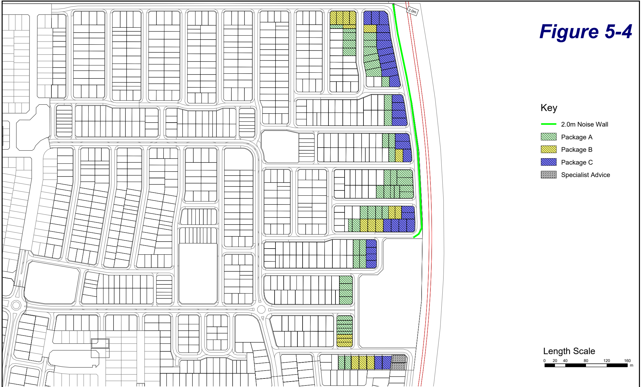
Ocean Hill North East Stages - Assuming 2.0m Noise Barrier Facade Treatment Packages - First Floor
